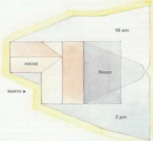
Winter shadows are much longer and can shift dramatically within the space of a few hours. Compare the shadow cast at noon to that cast at 2 pm.
