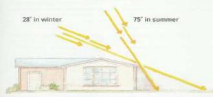
In winter, the sun crosses the sky at a lower angle than it does in summer. The effects can be pronounced, especially on north-facing exposures. The illustration above shows how the ground is shaded by the house at noon in summer and winter.
